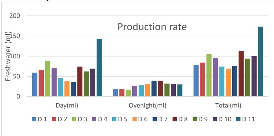
Figure 14. Comparison of daily freshwater production, overnight freshwater production, and total freshwater production
