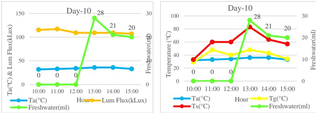
Figure 12(a), (b). Variation of hourly freshwater productivity with climatic factors & different temperatures for 9.4. 2023.
