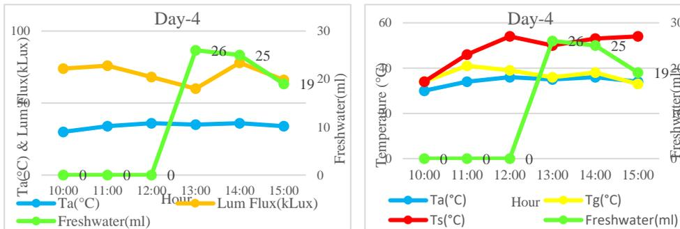
Figure 6(a), (b). Variation of hourly freshwater productivity with climatic factors & different temperatures for 3.4. 2023.
